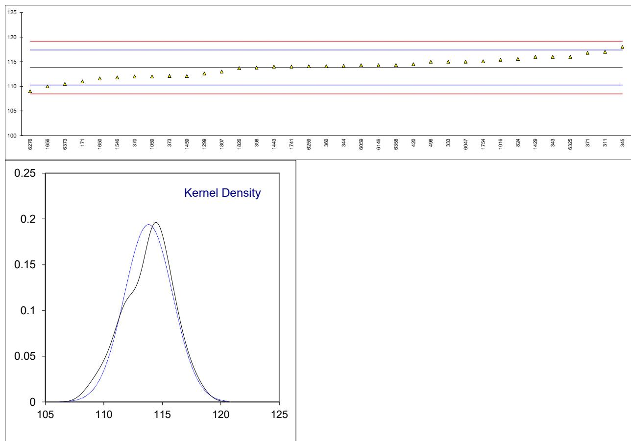
Determination of Kinematic Viscosity at 40 °C on sample #22205; results in mm<sup>2</sup>/s
