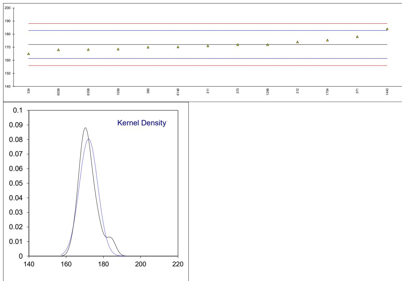
Determination of Iodine Value on sample #22205; results in g I<sub>2</sub>/100g
